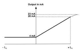
Note: 1) The performance specified in the datasheet is valid within the 4-20 mA output range only.
